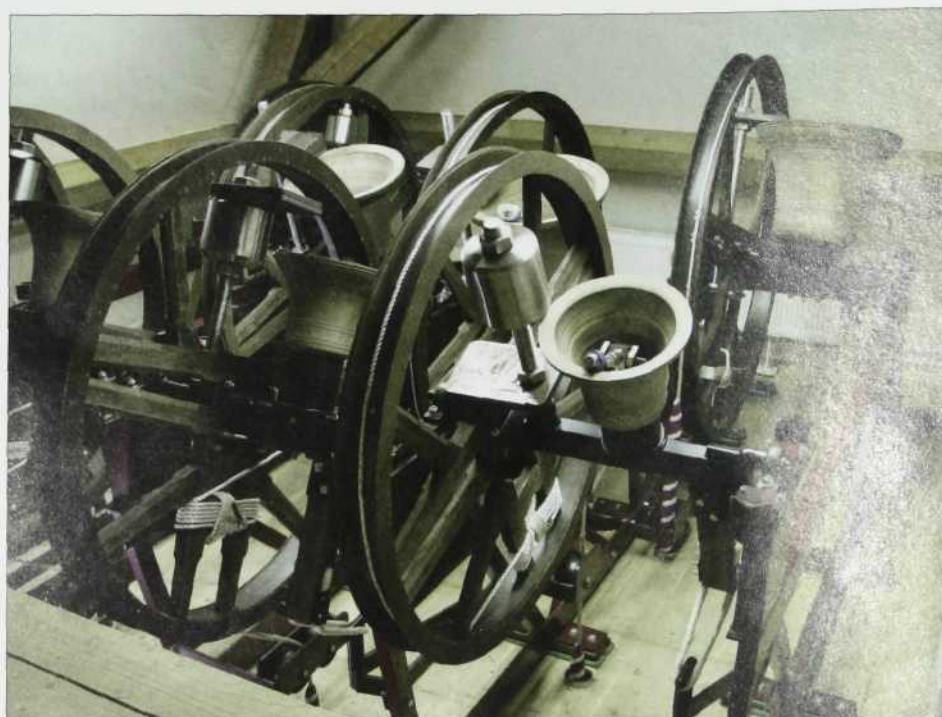
A close-up of the bells in the loft of the Klockhuys, showing the substantial weights on the small bells
